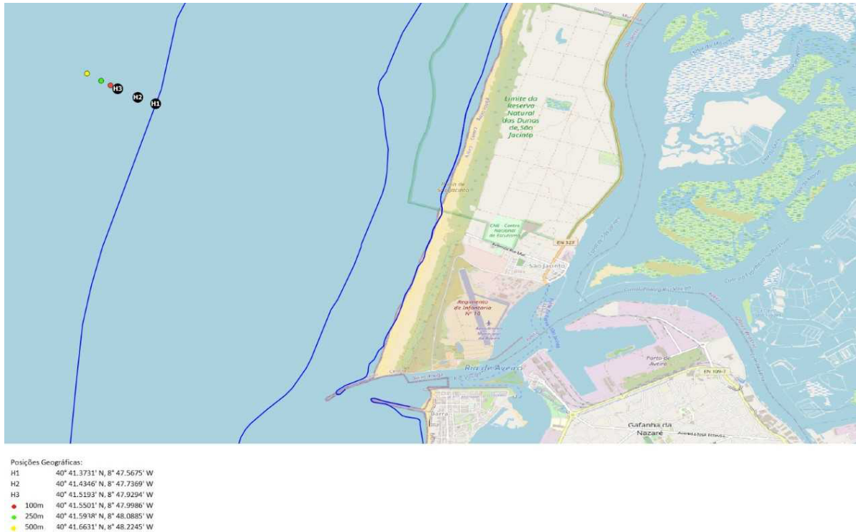
Figure 5.15: Configuration of the hydrophones and receptors for the second Aveiro campaign.
